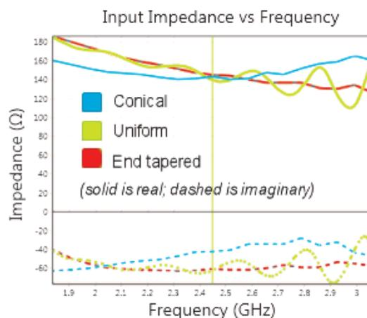
Comparison of the input impedances of three different types of helix antennas.
