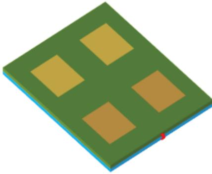
This patch array does not use a traditional feed network, but provides a nice practical way to achieve the higher gain and bandwidth that is possible with patch arrays without the need for an often sensitive and hard-to-design feed.
