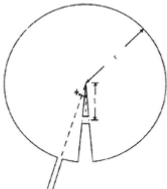
Diagram of the *Circular edge-fed patch with sectoral slot*.
