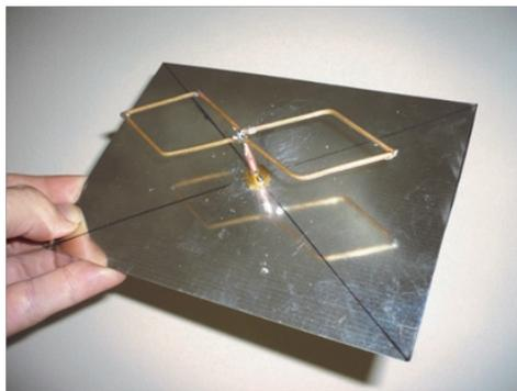
Photo of the Bi-Quad fabricated by the Antenna Magus engineers.
