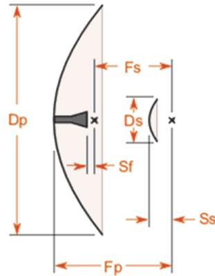
Side view of the Horn-fed Cassegrain reflector antenna.
