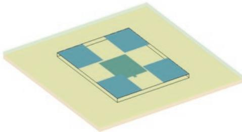
Transparent view of the *2x2 stacked patch array model*.
