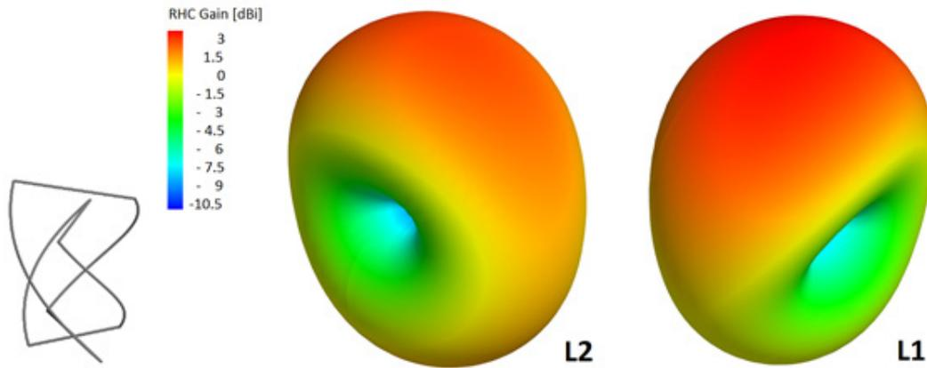
Radiation patterns of a dual-band self-phased quadrifilar helix antenna designed for GPS, at the L1 and L2 bands.
