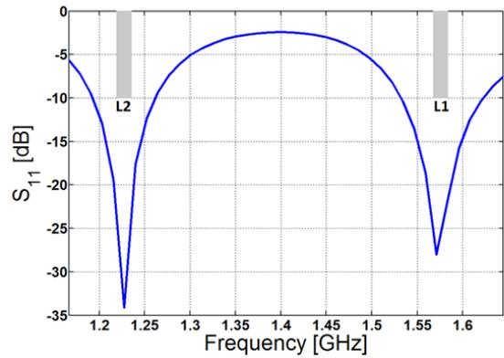
Reflection coefficient of a dual-band QHA designed for GPS, showing the operation in the L1 and L2 bands.
