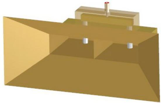
The structure of the short dual-waveguide fed horn antenna
