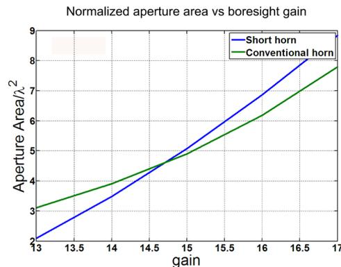
Comparison of the flare-length and aperture area of a conventional pyramidal horn and a dual-waveguide-fed horn, showing the shortened axial length required to achieve the same gain and aperture area for the dual-waveguide-fed horn.
