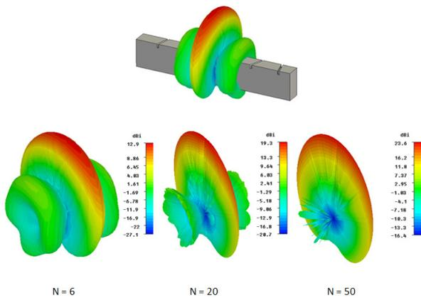
*Fan-beam radiation patterns of linear resonant narrow wall slotted guide arrays with 6, 20 and 50 elements respectively.*
