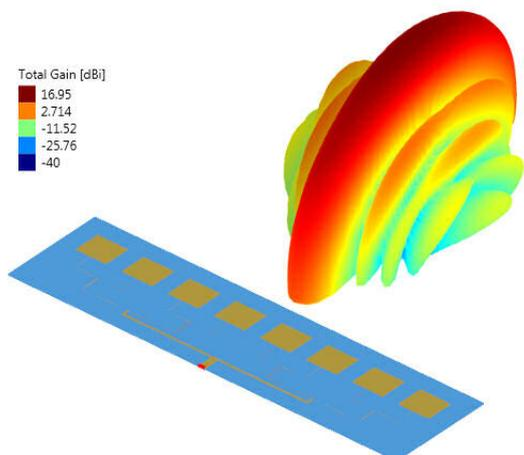
*The radiation pattern of an 8 element linear patch array with a corporate feed network*
