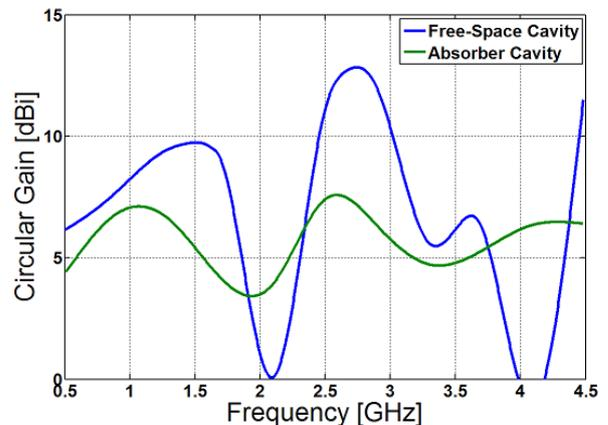
The boresight, circularly polarised gain vs frequency of a Sinuous antenna designed for 3:1 bandwidth from 1 - 3 GHz in free-space (a) placed above a free-space reflective cavity (b) above an absorbing cavity.
