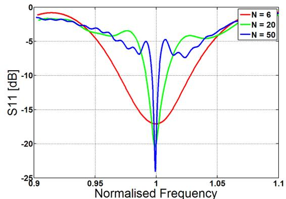
*Reflection coefficient performance of narrow wall resonant slot array normalised to the operating frequency, for 6, 20 and 50 slots*
