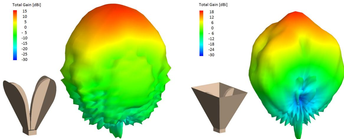
A comparison of the radiation patterns of dual-ridged horn with and without side walls, showing the reduction in beam splitting at the higher frequencies for the design without side walls.
